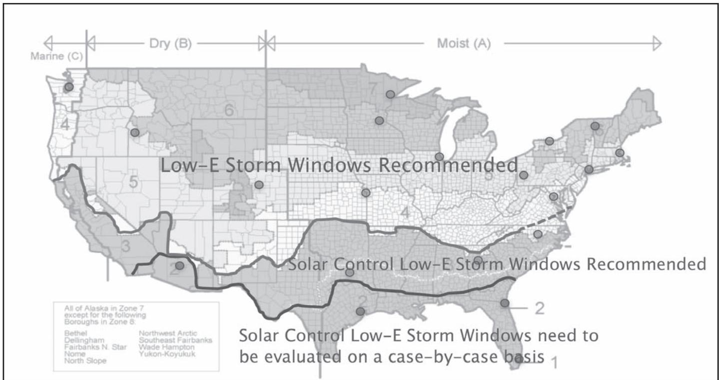
Figure 3. Cost effectiveness of Low-E storm windows across the US, by climate zone. Culp, TD, KA Cort. 2014. *Database of Low-E Storm Window Energy Performance Across US Climate Zones*. US DOE project #DE-AC05-76RL01830. Available online at [http://www.pnnl.gov/main/publications/external/technical\\_reports/PNNL-22864rev2.pdf](http://www.pnnl.gov/main/publications/external/technical_reports/PNNL-22864rev2.pdf).
