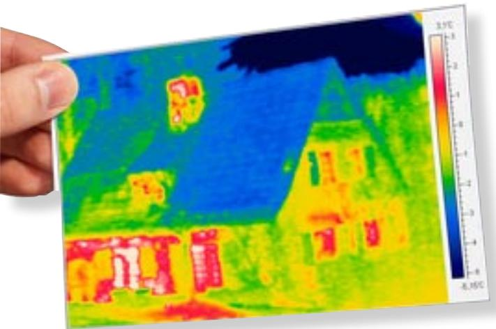
An infrared thermograph identifies sources of heat loss in this home. Red indicates zones of maximum heat loss. Images such as this can be used to identify where improvement is most needed.
